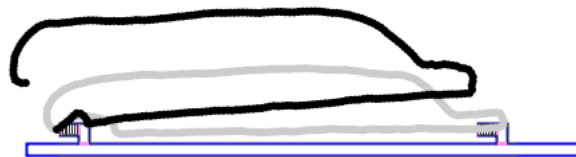
Figure 7. Two trials inside of a tunnel with small disturbances of the earth's magnetic field. The pedestrian passed the track in both directions.
